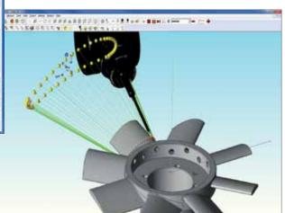
the inspection routine, performing the measurement and then evaluating the results can be up to 10 times faster than with typical aerofoil measurement software. Programming is intuitive and easy to use, with real-time evaluated results displayed graphically and numerically, with staggered-pitch blisks handled as easily as constant pitch designs.
